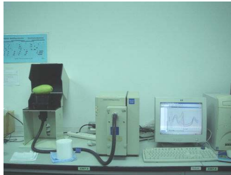
Figure 1 NIR instrument (NIRSystem6500) with fiber optic in interactance mode.
