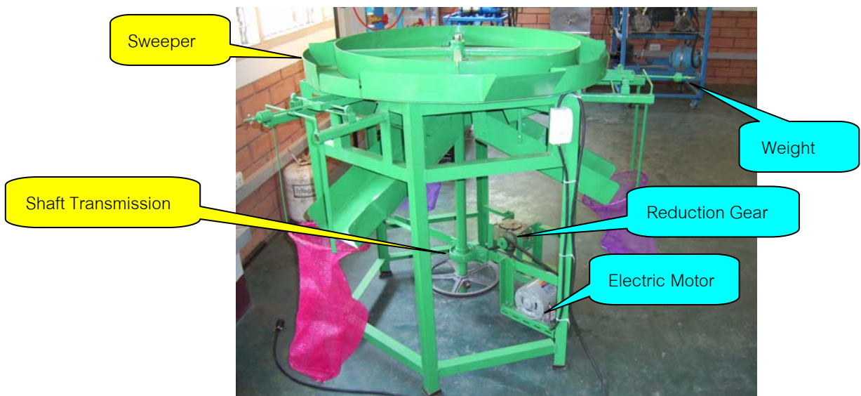
Figure 1 Consisting of Orange Grader by Weight Machine
