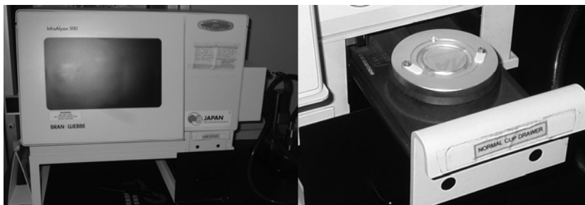
Figure 1 The NIR instrument and sample presentation of mangosteen juice.
