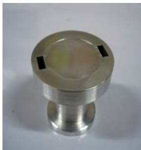
Figure 1 A specially designed sample cell for solution
