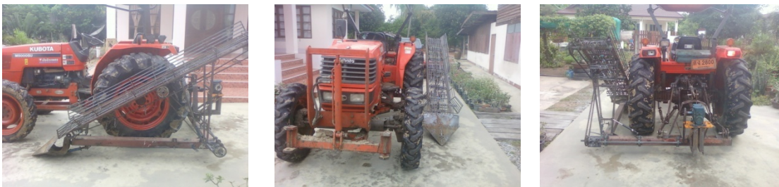
Figure 1 Cassava harvesting equipment for use on tractor
