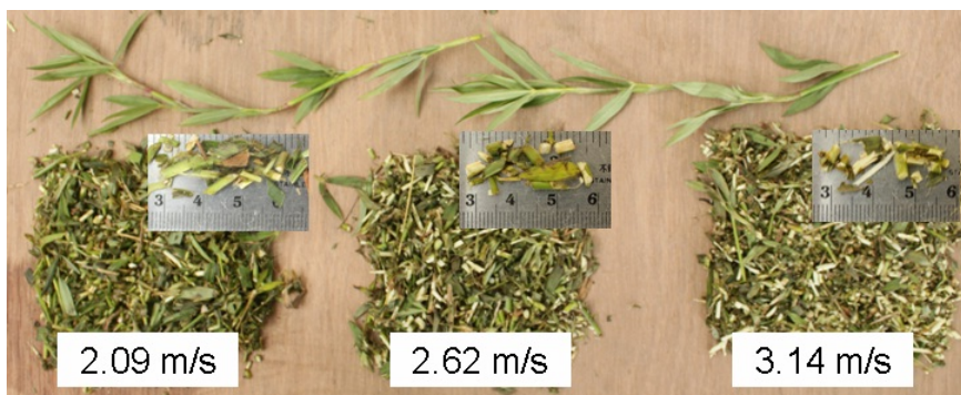
Figure 2 Sliced Thapra stylo bean at difference slicing disc speed
