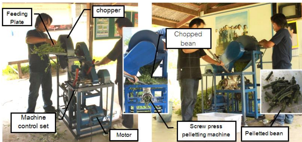
Figure 1 Prototype machine to produce the Thapra stylo bean pellet as feedstuff
