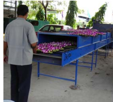
Fig2. Orchid moisture removal method with the prototype machine.
