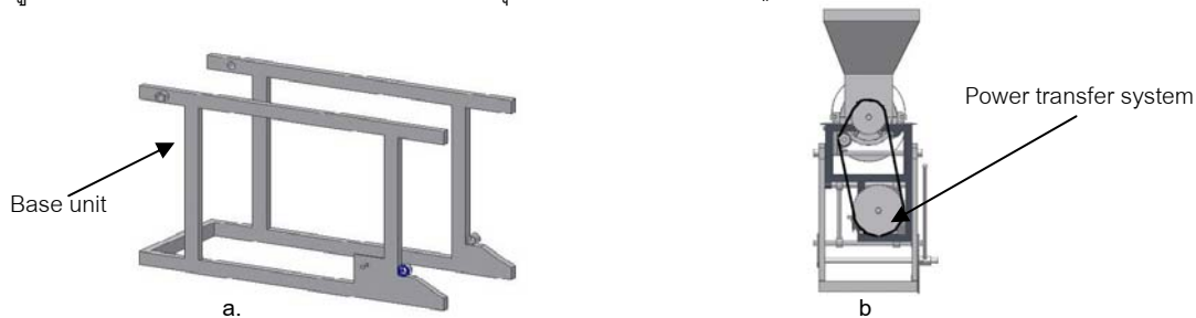
Figure 2 a. Base unit b. Power transfer system
