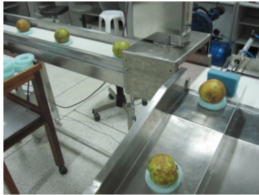
Figure 3 Automatic fruits sweetness grading system on conveyor
