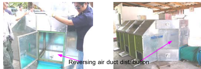
Fig. 1 Reversing air duct distribution system
