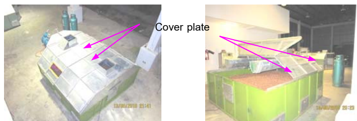
Fig. 3 Cover plate of modified batch dryer
