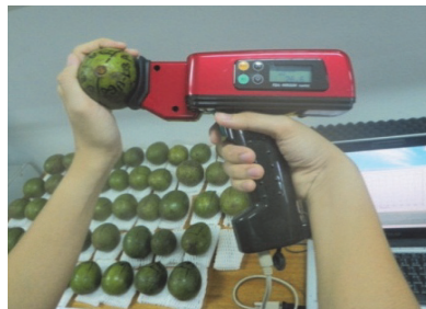
Figure 1 Spectra measurement using portable NIR Spectrometer (FQA-NIRGUN)
