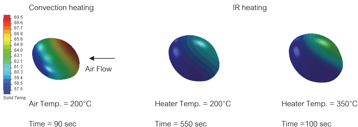
Figure 2 Soybean surface temperature (top view) under convection (left) and IR (middle and right) heating, at the same average surface temperature scale.
