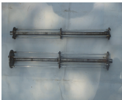
Figure 1 Sugar cane dry leaves removal mechanism
