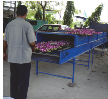
Figure 2. Orchid moisture removal method with the prototype machine
