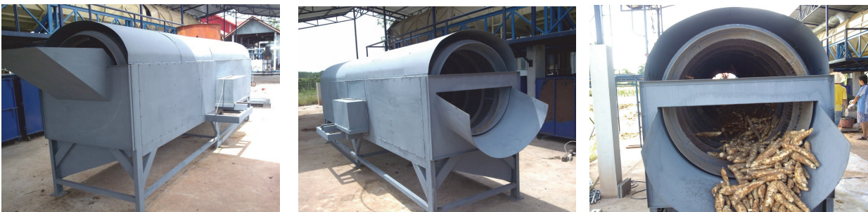
Figure 1 A trommel-type cassava cleaning machine
