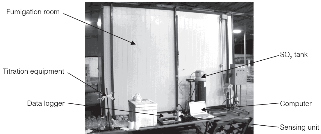
Figure 2 Field testing of SO 2 measuring device in 3x3x2.5 m 3 fumigation room.
